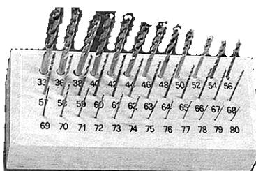
Set of 36 High Speed Steel Twist Drill
