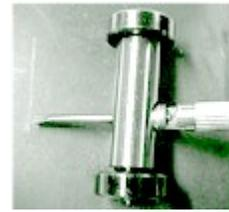
Spring action holds screwdriver firmly in place. Steel wheels are carefully set into body to provide even action when wheeled over stone. Overall width is 1-9/16.
