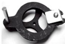
For Loop End mainsprings. Wind up On mainwheel and arbor from clock.
