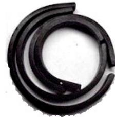
Set of 8 Flat Main Spring clamps Two Of each size. The two larger sizes made from flat steel 1/8" X 5/16. The two smaller sizes are made from 1/8" X 1/4" flat steel.
