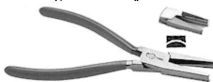
This large 6 1/2" German made ring Bending pliers has a box-joint with cushion grip handles for maximum leverage. Jaws are concaved/convex for shaping metal, with the convex jaw being slightly thinner than the concave jaw. Ground edges on the concave jaw minimize maring of precious metals. They can also be used to form mainspring end of clocks and etc..
