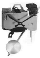
Shaft fits dials up to 5/16" Movement size is 7" High X 5-7/8" Wide By 2" Deep Takes A "D" battery (not included). Pendulum rod adjustable to 15-1/8" This movement will work With the pendulum or without pendulum. Mounting Hardware Included.
