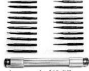
Set contains two each of 10 difference size hardened steel punches. Flat tips range from .020" to .050" in diameter and are easily ground to make other sizes. Punches are 1-5/8" long, with a 3/32" Shank. Used to drive out pins, broken Screws, riveting, etc.Brass holder 3-1/4" Long.
