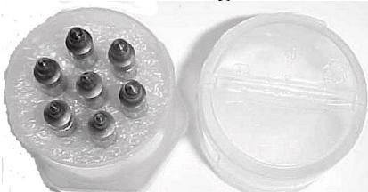
Used for reducing hole sizes in brass plates in Clocks, meters, etc. Spring center guides punch so that it will be concentric. Punch is tapped with small hammer.
